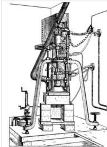
A sketch of an early furnace used by Verneuil to synthesise rubies using the Verneuil process
